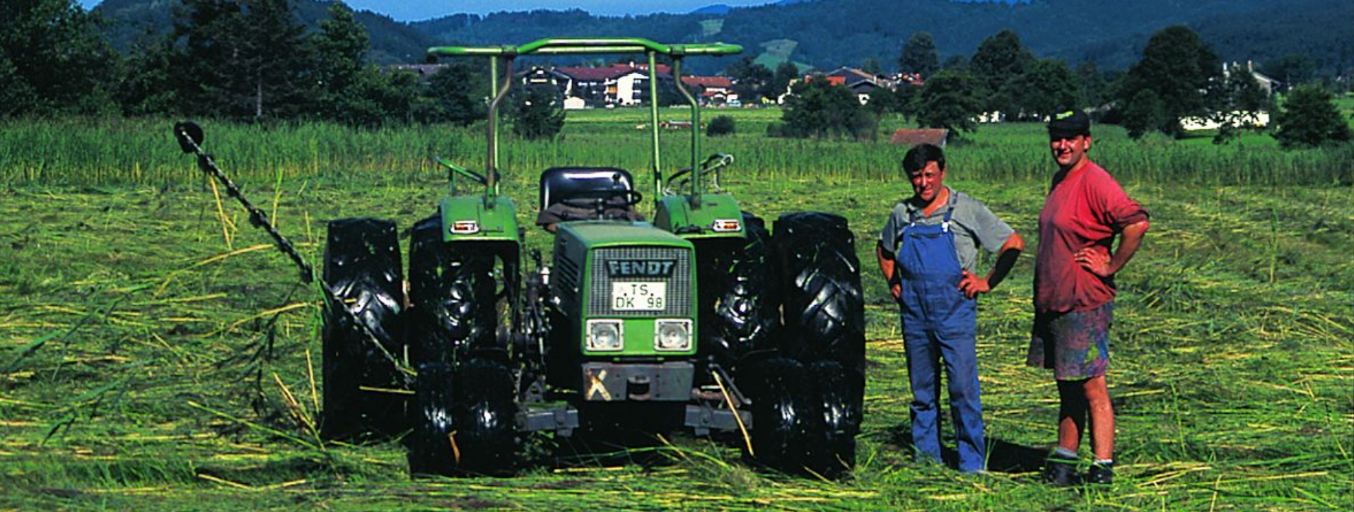
Light mowing-machine at the side, double twin wheels, 4wheel drive
